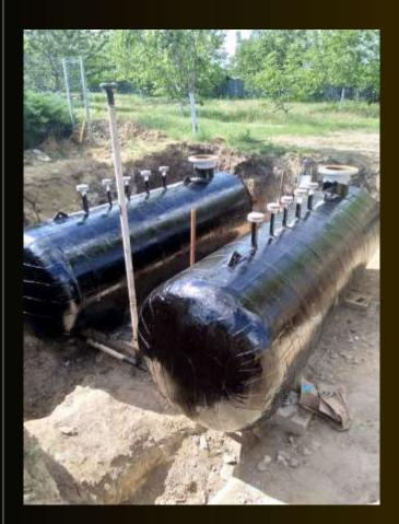
Storage capacities starting from 5 cubic meter to 250 cubic meter enable our customers to perform a flexible production, while high performance coating applications in accordance with EN 12944 ensure durability. With a new design of man-holes, we assist our clients save space during transportation.
