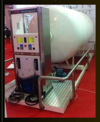
Skid LPG Systems are ideal to use in rural areas or for new businesses where low capacity is required. As the system is self-contained – i.e. a combination of storage tank and disposer or filling equipment with scales with all wiring and piping components installed within a 40 feet container size – there is no need for any type of construction. It is as easy and safe as to use just like Plug & Play computer equipment.
