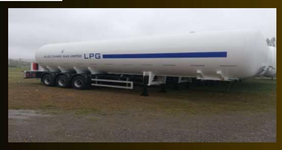
Used to transport relatively high amounts of LPG where high filling needs are present, semi-trailers should combine safety and efficiency needs of ground storage tanks with vehicle safety, operational reliability and low maintenance needs. Available from 38 m³ to 80 m³.
