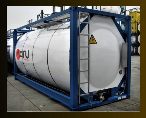
Designed to carry LPG in bulk like semi-trailers and bobtails, ISO tanks offer versatility for intermodal transportation where different modes of transport such as road, rail and/or sea needed combined to reach the final destination.
