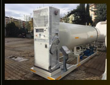
Skid LPG Systems are ideal to use in rural areas or for new businesses where low capacity is required. As the system is self-contained – i.e. a combination of storage tank and disposer or filling equipment with scales with all wiring and piping components installed within a 40 feet container size – there is no need for any type of construction. It is as easy and safe as to use just like Plug & Play computer equipment.
