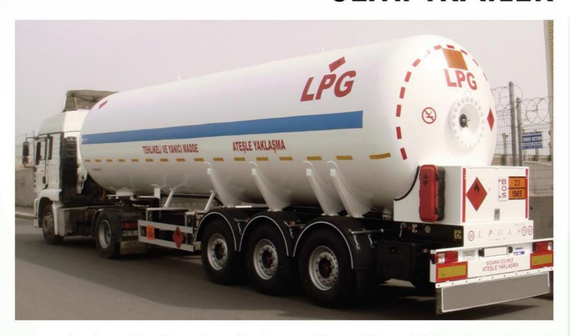
Designed and manufactured in the strength for cruising with a full load and road conditions. Trailers are manufactured in the form of a half frame, high-strength steel is used in frame.
