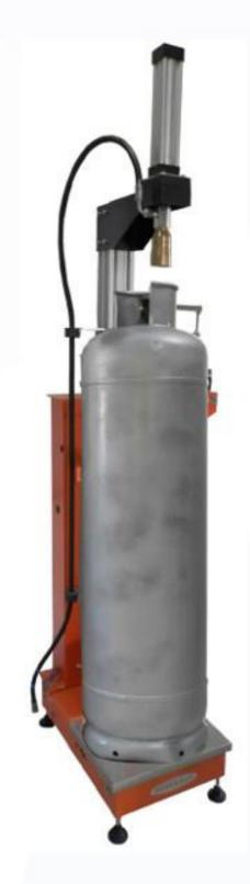
Used for domestic/industrial/camping, 2~50kg, all type lpg cylinders' filling.
