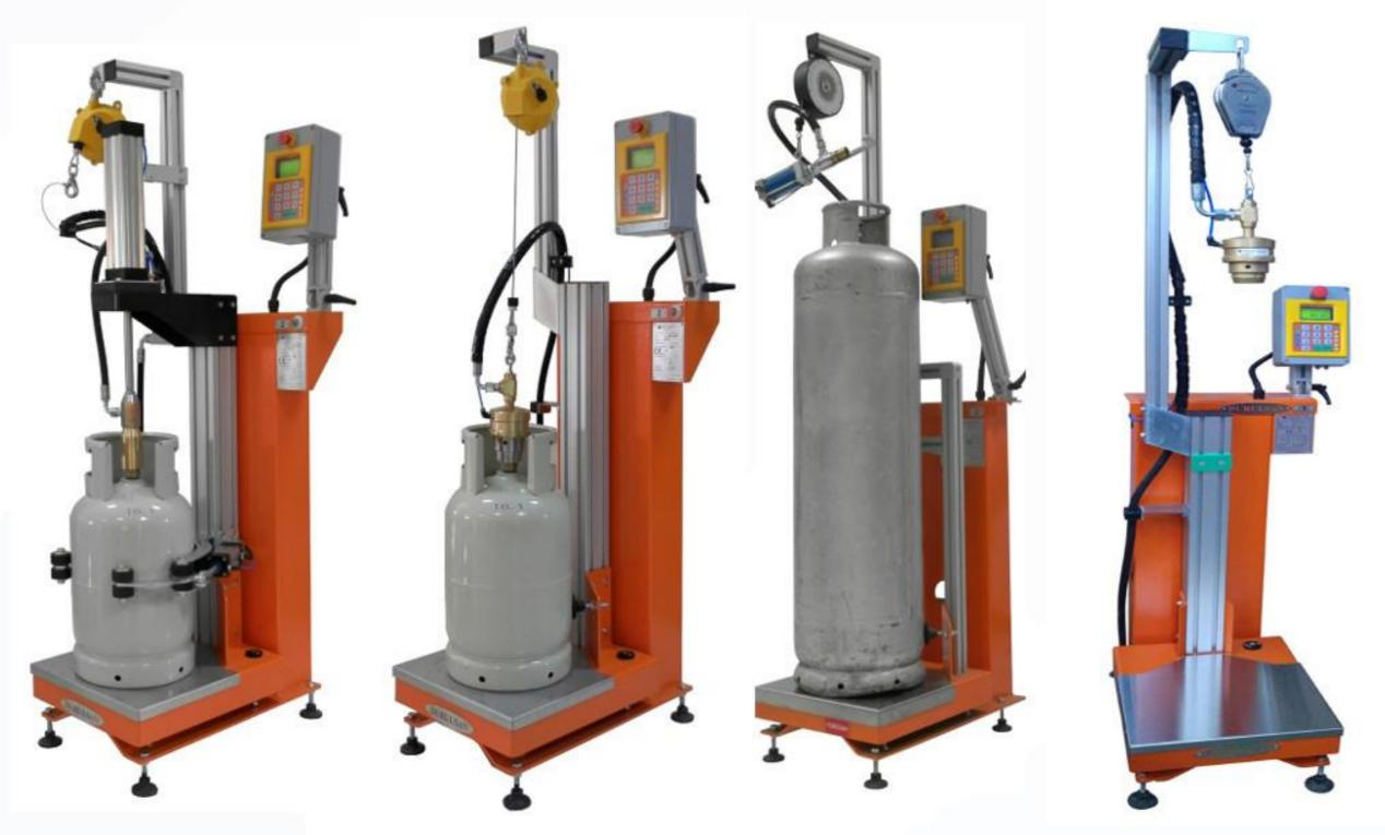
Used for domestic/industrial/camping 2~50kg, all type lpg cylinders' filling.
